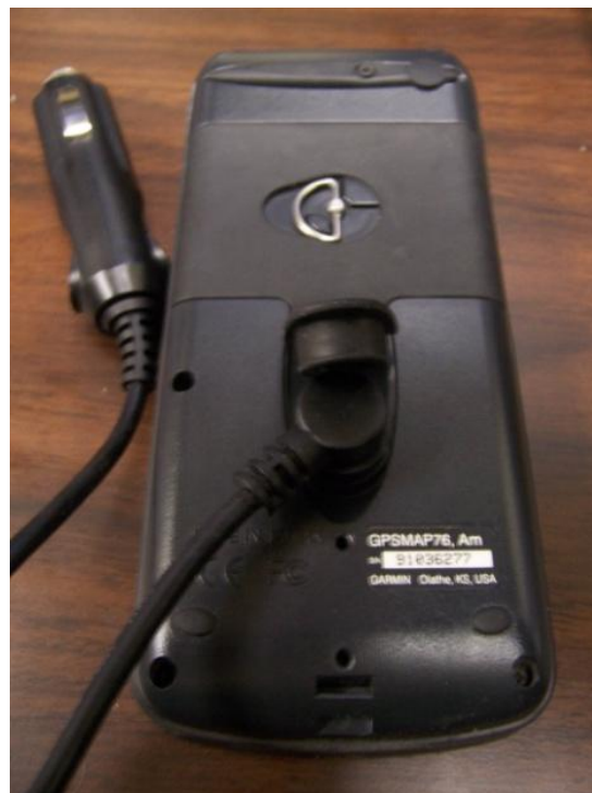
Figure 11: Powering the GPS Unit via Car Charger
